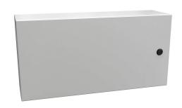
Hammond Eclipse series enclosure, NEMA 3R/4/12,  $12 \times 24 \times 6in$  (HxWxD), wall mount, carbon steel, RAL 7035 light gray, powder coat finish, single-door, 1/4-turn semi-flush latch.
