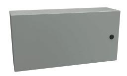
Hammond Eclipse series enclosure, NEMA 3R/4/12,  $12 \times 24 \times 6in$  (HxWxD), wall mount, carbon steel, ANSI 61 gray, powder coat finish, single-door, 1/4-turn semi-flush latch.
