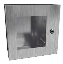
Hammond Eclipse series enclosure, NEMA 3R/4/4X/12/13,  $12 \times 12 \times 6$  in (HxWxD), wall mount, 304 stainless steel, #4 brush finish, single-door, 1/4-turn semi-flush 316 stainless steel latch, polycarbonate window.
