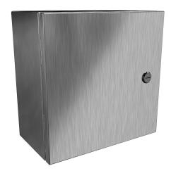
Hammond Eclipse series enclosure, NEMA 3R/4/4X/12/13, 12 x 12 x 6in (HxWxD), wall mount, 304 stainless steel, #4 brush finish, single-door, 1/4-turn semi-flush 316 stainless steel latch.
