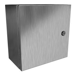
Hammond Eclipse series enclosure, NEMA 3R/4/4X/12/13, 12 x 12 x 6in (HxWxD), wall mount, 316 stainless steel, #4 brush finish, single-door, 1/4-turn semi-flush 316 stainless steel latch.
