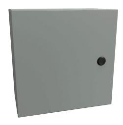
Hammond Eclipse series enclosure, NEMA 3R/4/12,  $12 \times 12 \times 6$ in (HxWxD), wall mount, carbon steel, ANSI 61 gray, powder coat finish, single-door, 1/4-turn semi-flush latch.
