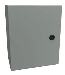
Hammond Eclipse series enclosure, NEMA 3R/4/12,  $12 \times 10 \times 6$ in (HxWxD), wall mount, carbon steel, ANSI 61 gray, powder coat finish, single-door, 1/4-turn semi-flush latch.
