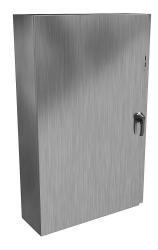
Hammond Eclipse series disconnect enclosure, NEMA 3R/4/4X/12/13, right flange, 60 x 38 x 12in (HxWxD), wall mount, 304 stainless steel, #4 brush finish, single-door, 3-point padlocking handle.
