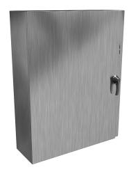
Hammond Eclipse series disconnect enclosure, NEMA 3R/4/4X/12/13, right flange, 48 x 38 x 12in (HxWxD), wall mount, 304 stainless steel, #4 brush finish, single-door, 3-point padlocking handle.
