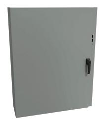
Hammond Eclipse series disconnect enclosure, NEMA 3R/4/12/13, right flange, 48 x 38 x 12in (HxWxD), wall mount, carbon steel, ANSI 61 gray, powder coat finish, single-door, 3-point padlocking handle.
