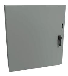
Hammond Eclipse series disconnect enclosure, NEMA 3R/4/12/13, right flange, 42 x 38 x 12in (HxWxD), wall mount, carbon steel, ANSI 61 gray, powder coat finish, single-door, 3-point padlocking handle.
