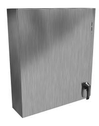
Hammond Eclipse series disconnect enclosure, NEMA 3R/4/4X/12/13, right flange,  $36 \times 32 \times 8$  in (HxWxD), wall mount, 304 stainless steel, #4 brush finish, single-door, 2-point padlocking handle.
