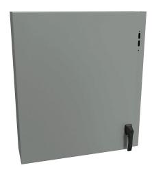
Hammond Eclipse series disconnect enclosure, NEMA 3R/4/12/13, right flange, 36 x 32 x 8in (HxWxD), wall mount, carbon steel, ANSI 61 gray, powder coat finish, single-door, 2-point padlocking handle.
