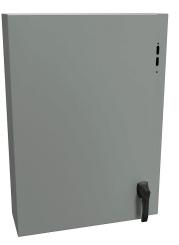
Hammond Eclipse series disconnect enclosure, NEMA 3R/4/12/13, right flange,  $36 \times 26 \times 8in$  (HxWxD), wall mount, carbon steel, ANSI 61 gray, powder coat finish, single-door, 2-point padlocking handle.
