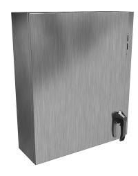
Hammond Eclipse series disconnect enclosure, NEMA 3R/4/4X/12/13, right flange,  $30 \times 26 \times 8$  in (HxWxD), wall mount, 304 stainless steel, #4 brush finish, single-door, 2-point padlocking handle.
