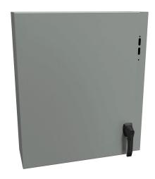
Hammond Eclipse series disconnect enclosure, NEMA 3R/4/12/13, right flange,  $30 \times 26 \times 8$  in (HxWxD), wall mount, carbon steel, ANSI 61 gray, powder coat finish, single-door, 2-point padlocking handle.
