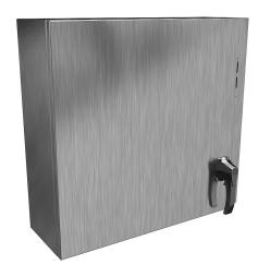
Hammond Eclipse series disconnect enclosure, NEMA 3R/4/4X/12/13, right flange,  $24 \times 26 \times 8$  in (HxWxD), wall mount, 304 stainless steel, #4 brush finish, single-door, 2-point padlocking handle.
