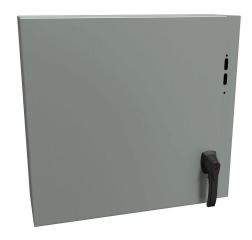
Hammond Eclipse series disconnect enclosure, NEMA 3R/4/12/13, right flange, 24 x 26 x 8in (HxWxD), wall mount, carbon steel, ANSI 61 gray, powder coat finish, single-door, 2-point padlocking handle.
