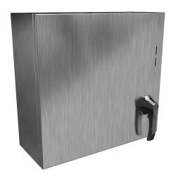
Hammond Eclipse series disconnect enclosure, NEMA 3R/4/4X/12/13, right flange, 20 x 22 x 8in (HxWxD), wall mount, 304 stainless steel, #4 brush finish, single-door, 2-point padlocking handle.
