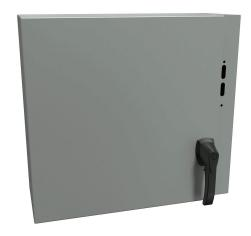
Hammond Eclipse series disconnect enclosure, NEMA 3R/4/12/13, right flange,  $20 \times 22 \times 8$  in (HxWxD), wall mount, carbon steel, ANSI 61 gray, powder coat finish, single-door, 2-point padlocking handle.
