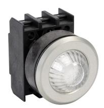
Schmersal illuminated indicating light, permanent light function, IP65, 30mm, white, 34.5mm, dome, plastic base, metal bezel. Requires light block and LED or incandescent bulb.
