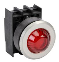
Schmersal illuminated indicating light, permanent light function, IP65, 30mm, red, 34.5mm, dome, plastic base, metal bezel. Requires light block and LED or incandescent bulb.
