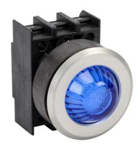
Schmersal illuminated indicating light, permanent light function, IP65, 30mm, blue, 34.5mm, dome, plastic base, metal bezel. Requires light block and LED or incandescent bulb.
