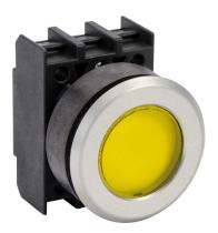
Schmersal illuminated indicating light, permanent light function, IP65, 30mm, yellow, 34.5mm, round, plastic base, metal bezel. Requires light block and LED or incandescent bulb.
