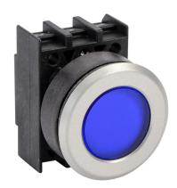
Schmersal illuminated indicating light, permanent light function, IP65, 30mm, blue, 34.5mm, round, plastic base, metal bezel. Requires light block and LED or incandescent bulb.
