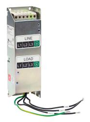
AutomationDirect EMI input filter, 480 VAC, 3-phase, 6A, panel mount, EMI/RFI filtering, drive rated, standard performance, screw terminals and ring terminals. For use with 3-phase GS10, GS20, GS20X and GS30 series AC drives.
