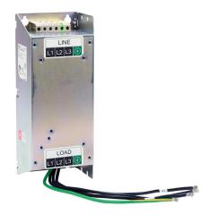
AutomationDirect EMI input filter, 240 VAC, 3-phase, 24A, panel mount, EMI/RFI filtering, drive rated, standard performance, screw terminals and ring terminals. For use with 3-phase GS10, GS20 and GS20X series AC drives.
