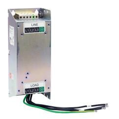
AutomationDirect EMI input filter, 240 VAC, 3-phase, 24A, panel mount, EMI/RFI filtering, drive rated, standard performance, screw terminals and ring terminals. For use with 3-phase GS10, GS20, GS20X and GS30 series AC drives.
