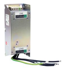
AutomationDirect EMI input filter, 480 VAC, 3-phase, 23A, panel mount, EMI/RFI filtering, drive rated, standard performance, screw terminals and ring terminals. For use with 3-phase GS10, GS20 and GS20X series AC drives.
