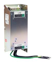
AutomationDirect EMI input filter, 600 VAC, 3-phase, 16A, panel mount, EMI/RFI filtering, drive rated, standard performance, screw terminals and ring terminals. For use with 3-phase GS20, GS20X and GS30 series AC drives.
