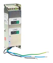
AutomationDirect EMI input filter, 240 VAC, 1-phase, 11A, panel mount, EMI/RFI filtering, drive rated, standard performance, screw terminals and ring terminals. For use with 1-phase GS10, GS20, GS20X and GS30 series AC drives.
