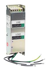
AutomationDirect EMI input filter, 240 VAC, 3-phase, 10A, panel mount, EMI/RFI filtering, drive rated, standard performance, screw terminals and ring terminals. For use with 3-phase GS10, GS20, GS20X and GS30 series AC drives.
