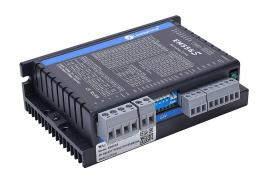
Leadshine DC microstepping stepper drive, 5.6A per phase, 2-phase output, 24-48 VDC, bipolar, position mode, 200 to 25600 steps per revolution.
