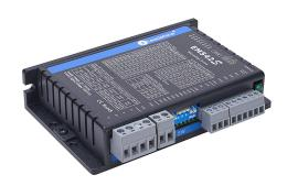
Leadshine DC microstepping stepper drive, 4.2A per phase, 2-phase output, 24-48 VDC, bipolar, position mode, 200 to 25600 steps per revolution.
