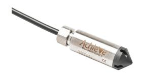
AchieVe hydrostatic submersible level transmitter, 0 to 50 psig (115.5ft of water column) sensing range, 4-20 mA, 0.825in diameter housing, shielded and vented 140ft cable.
