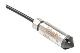
AchieVe hydrostatic submersible level transmitter, 0 to 15 psig (34.6ft of water column) sensing range, 4-20 mA, 0.825in diameter housing, shielded and vented 60ft cable.
