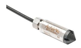
AchieVe hydrostatic submersible level transmitter, 0 to 5 psig (11.5ft of water column) sensing range, 4-20 mA, 0.825in diameter housing, shielded and vented 30ft cable.
