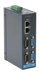
Advantech Modbus gateway, serial Master/Slave and Ethernet Client/Server, (2) Ethernet 10/100Base-T (RJ45) and (4) RS-232/422/485 (9-pin D-sub male) port(s), (64) simultaneous Ethernet connections, (128) serial device(s), 12-48 VDC required.
