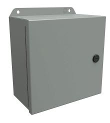
Hammond Eclipse Junior series enclosure, NEMA 3R/4/12/13, 8 x 8 x 4in (HxWxD), wall mount, carbon steel, ANSI 61 gray, powder coat finish, single-door, 1/4-turn semi-flush latch.
