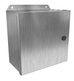
Hammond Eclipse Junior series enclosure, NEMA 3R/4/4X/12/13, 8 x 8 x 4in (HxWxD), wall mount, 304 stainless steel, #4 brush finish, single-door, 1/4-turn semi-flush 316 stainless steel latch.
