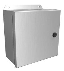
Hammond Eclipse Junior series enclosure, NEMA 3R/4/4X/12/13, 8 x 8 x 4in (HxWxD), wall mount, 5052-H32 aluminum, singledoor, 1/4-turn semi-flush 316 stainless steel latch.
