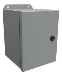
Hammond Eclipse Junior series enclosure, NEMA 3R/4/12/13, 8 x 6 x 6in (HxWxD), wall mount, carbon steel, ANSI 61 gray, powder coat finish, single-door, 1/4-turn semi-flush latch.
