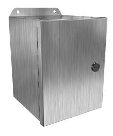
Hammond Eclipse Junior series enclosure, NEMA 3R/4/4X/12/13,  $8 \times 6 \times 6$  in (HxWxD), wall mount, 304 stainless steel, #4 brush finish, single-door, 1/4-turn semi-flush 316 stainless steel latch.
