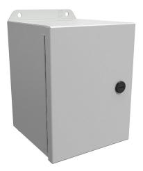
Hammond Eclipse Junior series enclosure, NEMA 3R/4/12/13, 8 x 6 x 6in (HxWxD), wall mount, carbon steel, RAL 7035 light gray, powder coat finish, single-door, 1/4-turn semi-flush latch.
