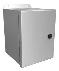
Hammond Eclipse Junior series enclosure, NEMA 3R/4/4X/12/13, 8 x 6 x 6in (HxWxD), wall mount, 5052-H32 aluminum, singledoor, 1/4-turn semi-flush 316 stainless steel latch.
