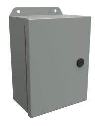
Hammond Eclipse Junior series enclosure, NEMA 3R/4/12/13, 8 x 6 x 3in (HxWxD), wall mount, carbon steel, ANSI 61 gray, powder coat finish, single-door, 1/4-turn semi-flush latch.
