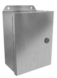
Hammond Eclipse Junior series enclosure, NEMA 3R/4/4X/12/13, 8 x 6 x 3in (HxWxD), wall mount, 316 stainless steel, #4 brush finish, single-door, 1/4-turn semi-flush 316 stainless steel latch.
