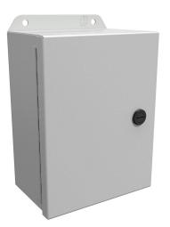
Hammond Eclipse Junior series enclosure, NEMA 3R/4/12/13, 8 x 6 x 3in (HxWxD), wall mount, carbon steel, RAL 7035 light gray, powder coat finish, single-door, 1/4-turn semi-flush latch.
