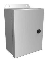
Hammond Eclipse Junior series enclosure, NEMA 3R/4/4X/12/13, 8 x 6 x 3.5in (HxWxD), wall mount, 5052-H32 aluminum, singledoor, 1/4-turn semi-flush 316 stainless steel latch.
