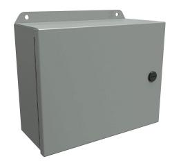
Hammond Eclipse Junior series enclosure, NEMA 3R/4/12/13, 8 x  $10 \times 4$  in (HxWxD), wall mount, carbon steel, ANSI 61 gray, powder coat finish, single-door, 1/4-turn semi-flush latch.
