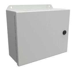
Hammond Eclipse Junior series enclosure, NEMA 3R/4/12/13, 8 x 10 x 4in (HxWxD), wall mount, carbon steel, RAL 7035 light gray, powder coat finish, single-door, 1/4-turn semi-flush latch.
